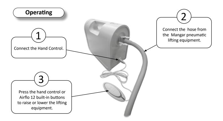
**IMPORTANT:** The Airflo 12 is designed not to deflate if there is insufficient battery voltage to fully inflate the lifting product. This safety feature stops an inflatable bathing product from being lowered to the bottom of a bath if there is insufficient battery voltage to raise it again.
