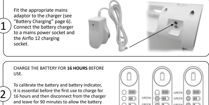
For the first 6 hours, the bottom light will flash green. After 6 hours the first light will become a steady green and the second light will start flashing. Charging cycle continues until lights are lit. Then after 16 hours the charge is complete with the top light flashing and other 3 will be off.
