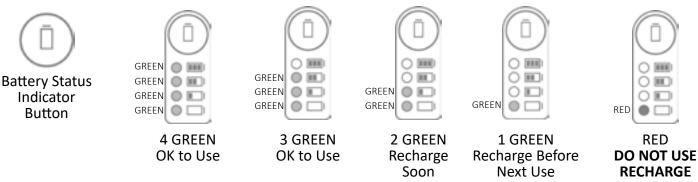
**WARNING**: The battery must be put on charge immediately as soon as the red indicator light appears. Running the Airflo 12 on RED until the battery is exhausted will damage the battery.
