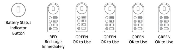
**NOTE:** The battery must be put on charge immediately as soon as the red indicator light appears. Running the Airflo 12 on RED until the battery is exhausted will damage the battery.
